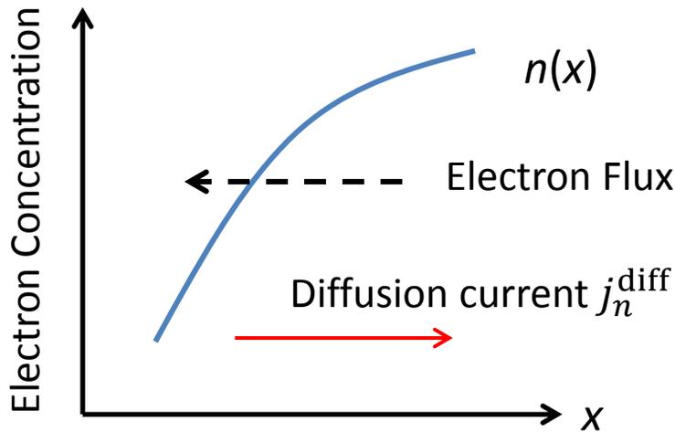
Electron flux:  $F_n = -D_n \frac{dn}{dx}$
